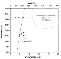
Apparatus for diamond synthesis and pressure-temperature graph that shows the parameters needed for the synthesis of high-purity diamonds.
